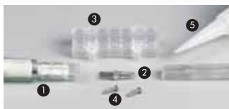
Front Connector 1. Shell electrical plug end 2. Simple front connector 3. Plastic Shell (2 Piece) 4. Self-tapping Screws 5. Silicone Adhesive
